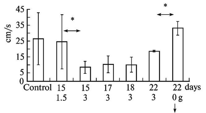
**Fig. 5.** Rate of cockroach movement on horizontal plane with load of 3.0 g. *Abcissa*: days of recording and weight of the load (g), *ordinate*: rate of movement (cm/s). Arrow—removal of the load. Asterisk indicates statistically significant differences at addition and removal of the load— $p < 0.05$ .
