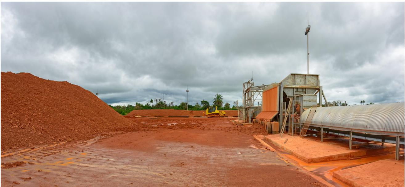
A covered conveyor belt mechanism transports bauxite ore, which is refined into aluminum, from an outside storage area to a bulk carrier. (Shutterstock)
